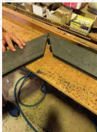
Step 3. Insert the Butt joiners as supplied.
