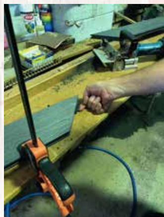
Step 2. Biscuit cut on both faces. Be sure the cut height is equal to bottom of board.
