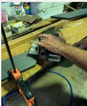
Step 1. Biscuit cut on both faces. Mark both tops with chalk as seen in step 4.
