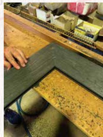
Step 4. Check to see the boards are even on all faces and they line up before you fix one of them.
